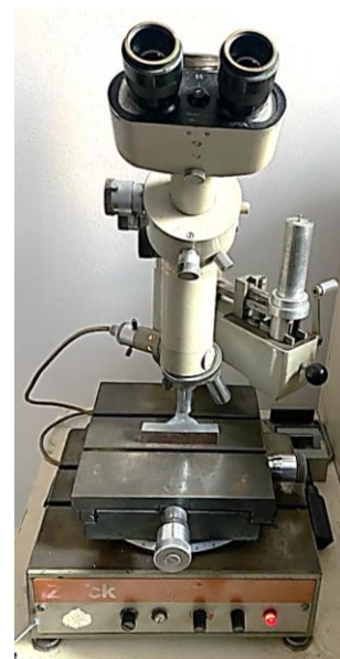
Figure 2. Zwick 3212 Hardness equipment
